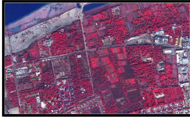
Figure 1 A false color composite in the Red, Near Infra-Red and Green bands with vegetation shown in red color variations.
